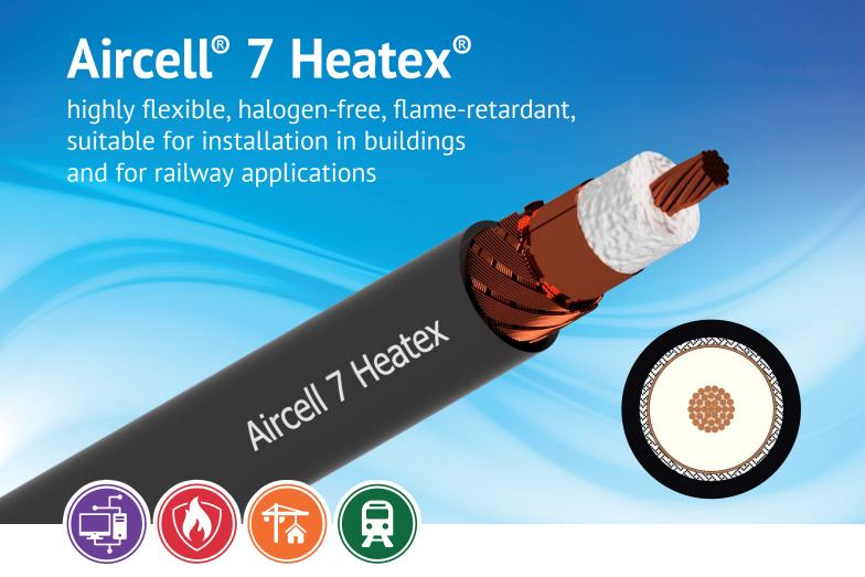
Aircell 7 Heatex is an ultraflexible coaxial cable designed for frequencies up to 6 GHz. Due to its low loss in relation to the outer diameter and the small bending radius the cable can be used for numerous RF applications.
